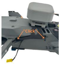
Swivel it slightly to "clip" the bracket into the drone's holes.
