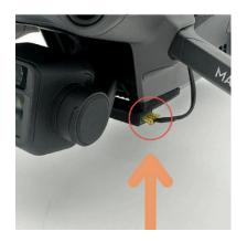
The parachute is now in place, so connect the system to the drone.
