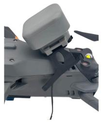
Attach the parachute to the drone
