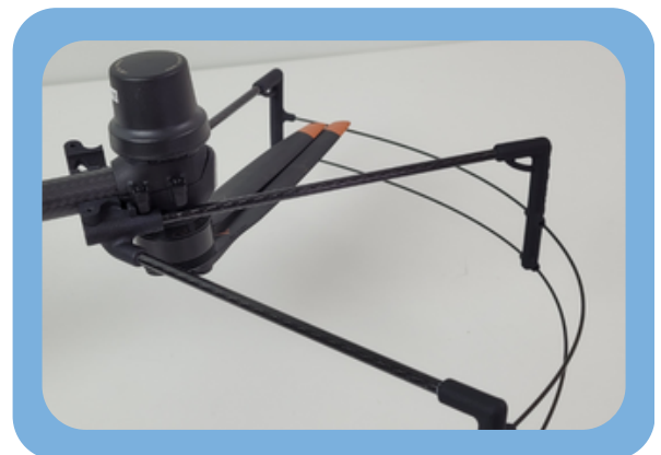
Insert propeller guard from below
