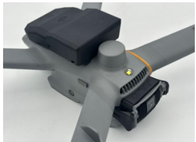
FTS/Parachute and geofencing are operated from the Standalone remote control on the ground. It is fitted to the drone's remote control and communicates with the receiver via a dedicated channel (868MHz) independent of those used by the drone.
