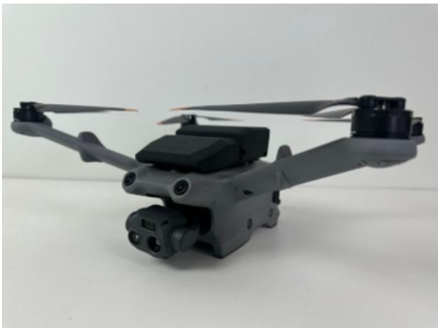
*Pic.2: Receiver and parachute attached to Matrice 3.*
