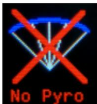
Indicates that the pyrotechnic charges are not connected. Please check parachute assembly.
