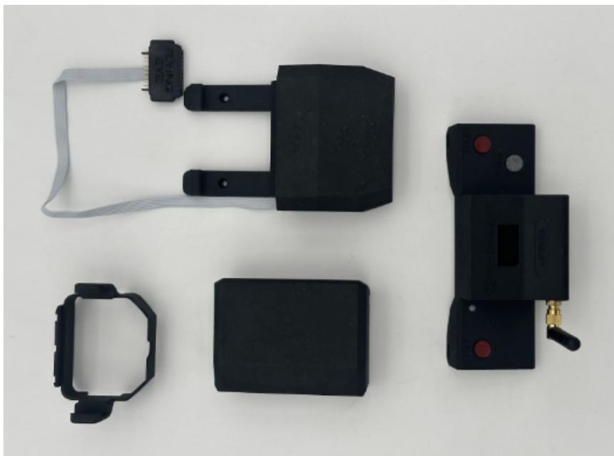
*Pic.1: FTS/Parachute system component with Geofencing for Matrice 3 (version 1).*
