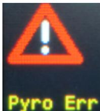
If the pyrotechnic charges are damaged or incorrectly connected, they must be inspected and the assembly checked.
